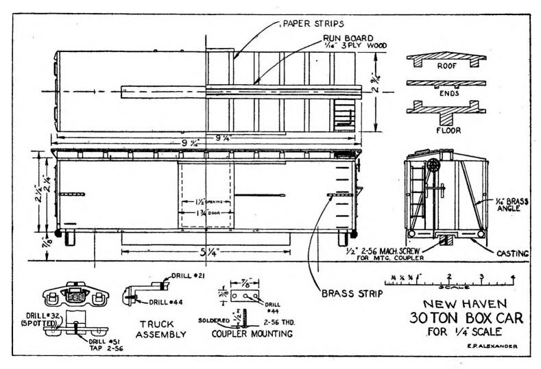
The end pieces with push-pole sockets are aluminum castings and may be nailed on with brads. The plates used for mounting couplers (usable for other cars as well) may be purchased or built up as shown in the drawing. Couplers should be drilled with No. 44 drill for mounting on these; nuts, of course, holding them on.
